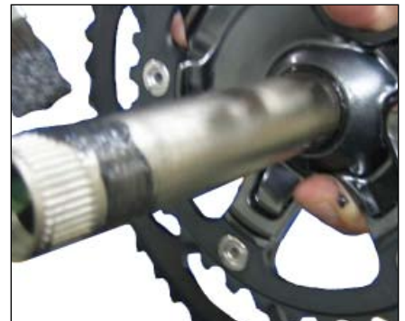
Figure 34. Greasing the axle
